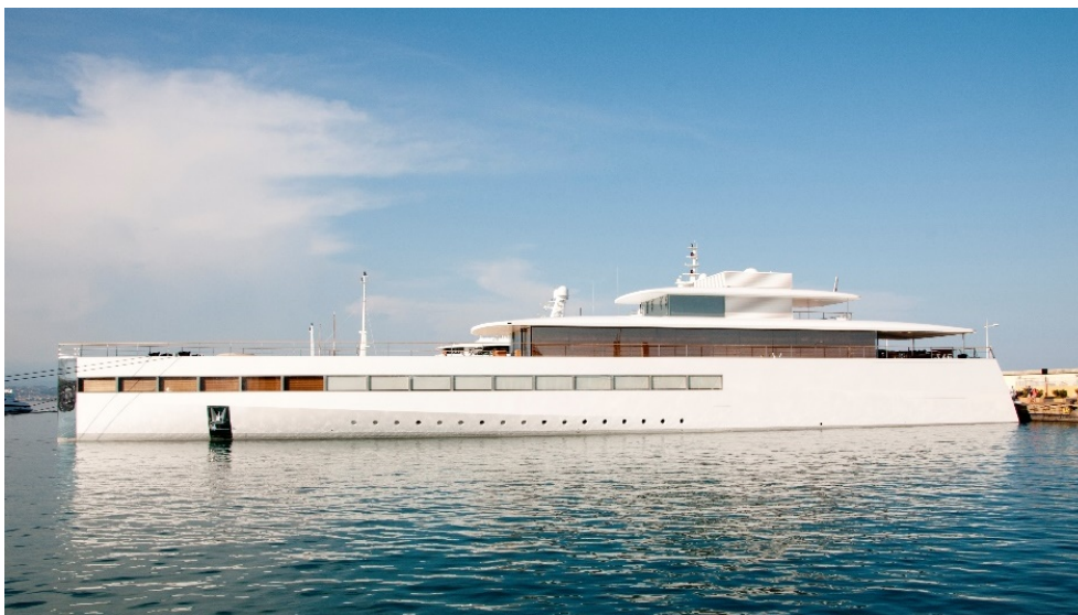
Fig. 1 Venus is one of the first superyachts in which glass was used extensively. Designer: Philippe Starck | Structural Glass Engineers: Eckersley O'Callaghan | Shipyard: Feadship Aalsmeer
